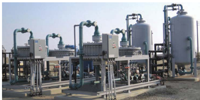
Produced water treatment system in Maricopa, California, with Spectrum Plus Micro-Media Filters and RecoPur SAC/WAC Ion Exchange Softeners.
